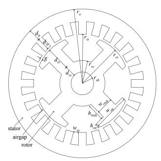
Fig. 7. Example WRSM configuration.
