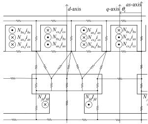
Fig. 8. Example WRSM MEC, including phase and field windings.
