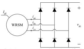
Fig. 9. System IV. WRSM with passive rectifier.
