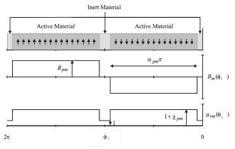
Fig. 4. Developed diagram of permanent magnet region.
