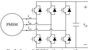
Fig. 2. System I. PMSM with active rectifier.
