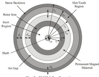
Fig. 3. PMSM Configuration.
